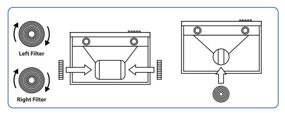
4. To replace the filter, rotate it counterclockwise and then remove it. After that, install the new charcoal filter and twist it clockwise to lock it in place.
