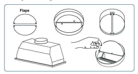
12. Connect the 6" round aluminum duct exhaust hose to the damper by placing one end of the hose over the flap and securing it with two small screws. Then, wrap the connection with tape or use a hose clamp and wrap it with tape to ensure a tight seal. Ensure that the circular damper is correctly positioned in the duct opening of the range hood and confirm its proper installation. Pull the ductwork and electrical cord through the cabinet hole.
