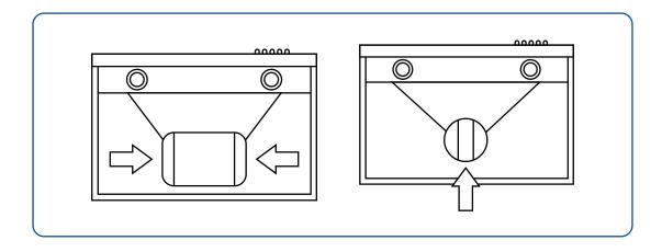
3. Take one filter and attach it to the motor. Rotate and twist it clockwise until it locks in place. If your range hood model calls for two filters to be installed, then the filters should be installed on each side. Repeat the previous step by taking another charcoal filter and attaching it to the other side of the motor. Rotate and twist it clockwise until it locks in place.
