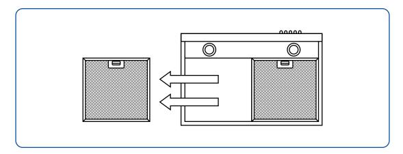
2. The placement of the charcoal filter varies depending on the model. In some models that only require I charcoal filter, the opening is in the middle of the motor. For models that require 2 charcoal filters, the openings are positioned on the sides of the motor. If you have any inquiries regarding the specific model that you have purchased, please don't hesitate to contact our support team.
