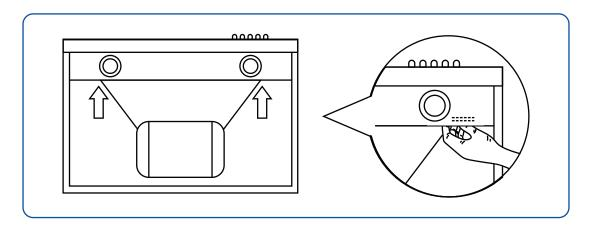
4. The wires for the LED lights are connected using a snap-down connector. To disconnect the LED lights, press down on the connector and gently pull the opposing electrical wire away from the connector.
