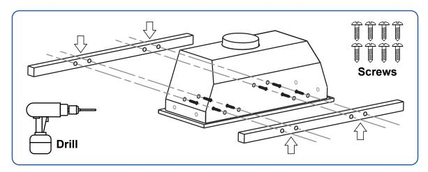
17. Additional support is recommended. There are 4 holes [2 on each side] located on the sides of the range hood specifically for fastening it to the side stud support. This will provide additional support for the range hood.
